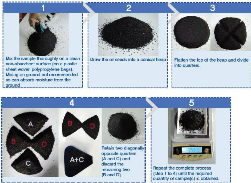
Figure 4 Coning and Quartering sampling method
